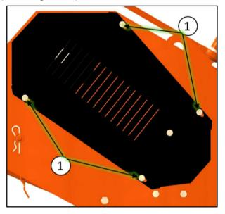
Once the cover has been removed, to check that the belt tension is correct, apply a force of approx. 10-15kg in the middle of the belts (halfway between the two pulleys) and measure the deflections (see image below)
