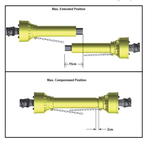
When shortening a PTO shaft, please note that you must shorten both the male and the female transmission shafts as well as BOTH covers. If the safety cover is removed (to facilitate shortening the shaft) it MUST be refitted so you comply with Health and Safety protocols.
