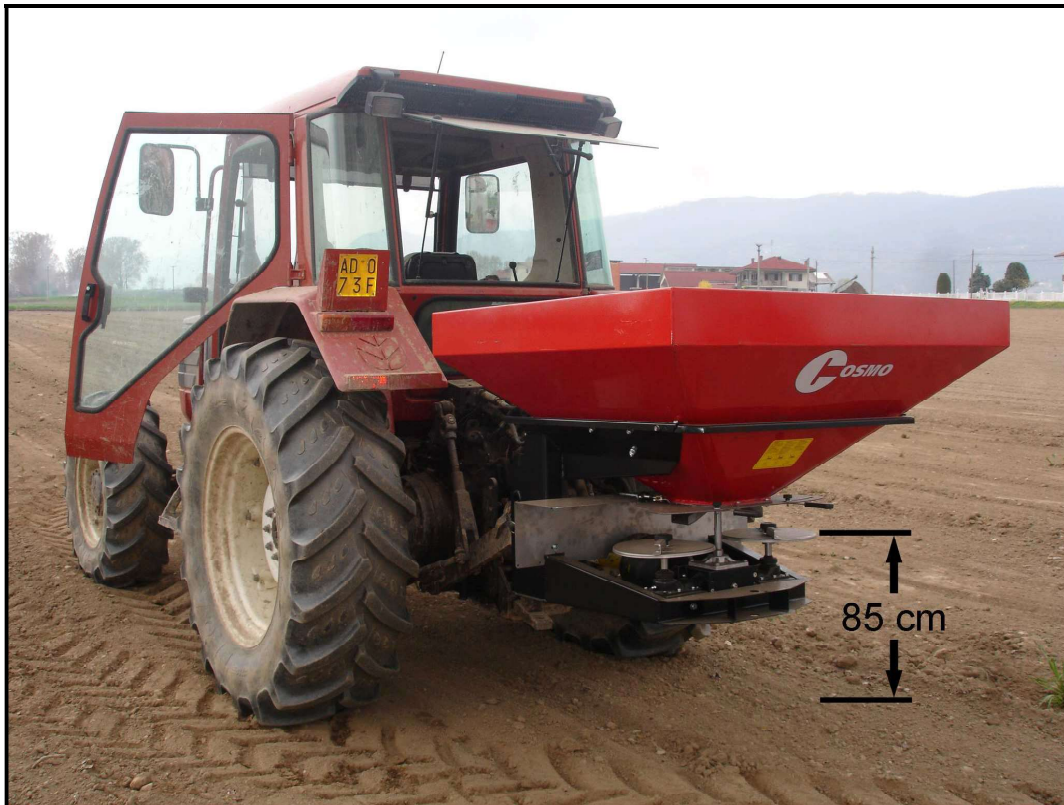
85 cm between the ground level and the distribution disc height
