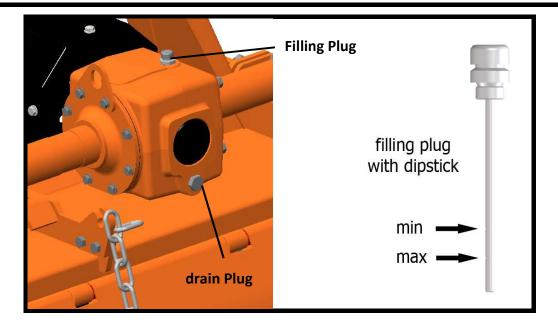
If the oil is below the minimum, fill up to restore the correct level.
