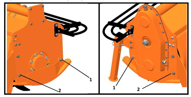
When finished, verify that both skids are at same level, and check if the front of the implement is levelled to the back, when lowered to the ground. Adjust with the 3-point top link if necessary.
