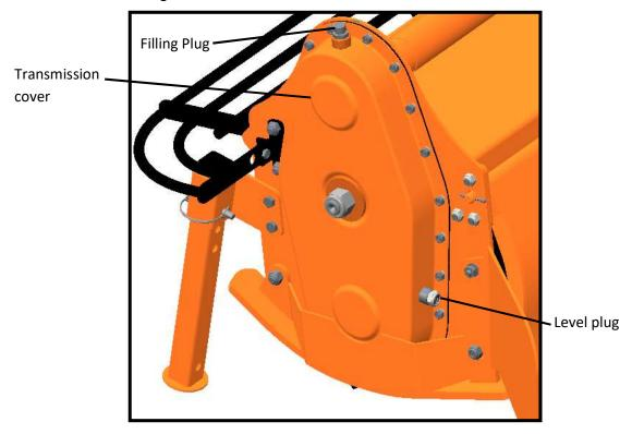
Check the oil level every 50 hours. Make sure it reaches the level plug on the transmission cover.
