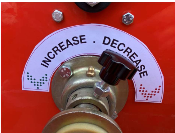
Figure 1. Front Seed Box adjustment direction(s)
