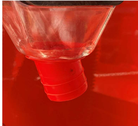
Figure 4. Seed Tube removed from Disc opener ready for plastic bag or container to capture material
