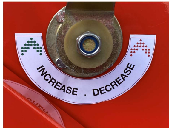
Figure 2. Rear Seed Box adjustment direction(s)
