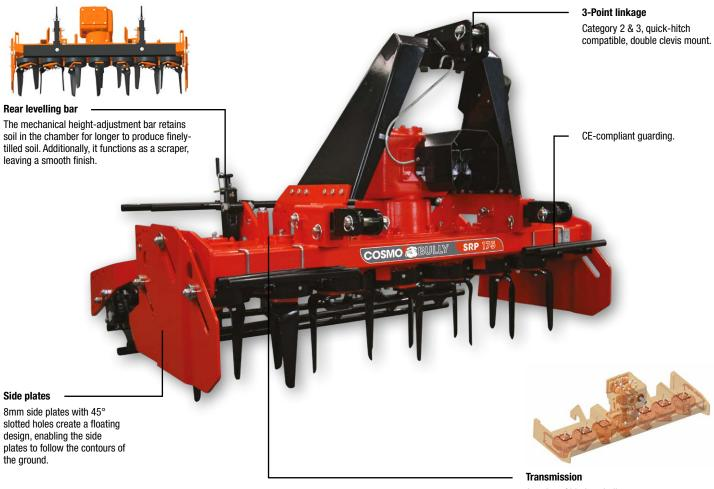
A series of blade spindles counter-rotate on a vertical axis, with gears aligned horizontally for maximum contact and power transfer between blade spindles.
