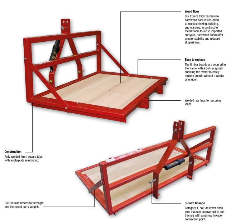
**KCWF150** Code **KCWF120 KCWF180** 1.2m | 4'0' 1.8m | 6'0' Size reference 1.5m | 5'0" Max. carry weight (kg) 600 750 900 Dimensions overall 1240 | floor 1200 overall 1540 | floor 1500 Width (mm) overall 1840 | floor 1800 Depth (mm) overall 1060 | floor 870 overall 1180 | floor 990 Weight (kg) 53 68 85
