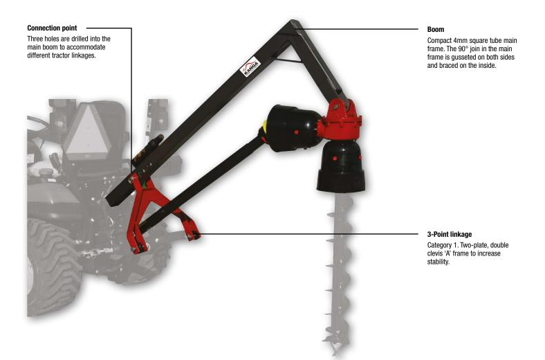
Australian-made and sold separately, the double-cut augers are 1.2m in length and, ground conditions permitting, result in hole depths of up to 1.1m. The augers have a replaceable cast-steel fishtail pilot and cast knock-in teeth# for faster, more efficient digging.
